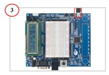
Connect the USB cable. LED5 lights up. The message "PSoC Eval USB 1" is displayed on the LCD. Observe that the mouse pointer on the PC screen moves in a square fashion.
